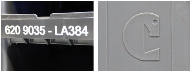
Lettering or sequential numbering (hot stamping) Injection-moulded logo
